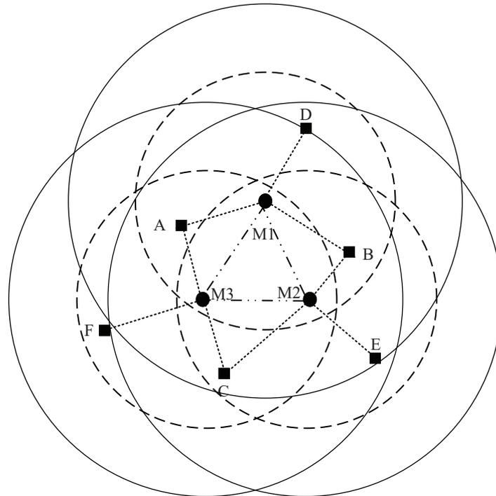
FIGURE 1. Schematic diagram of WSN node location based on RSSI
