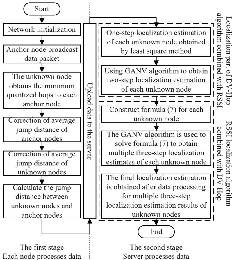
FIGURE 2. Schematic diagram of the overall architecture of the algorithm
