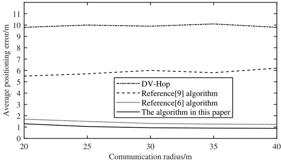
FIGURE 5. Variation curve of average localization error with communication radius
