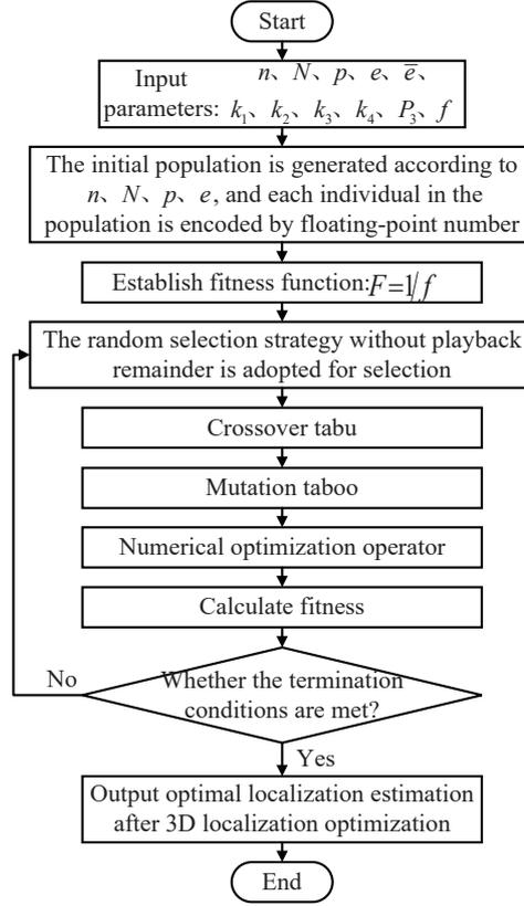
FIGURE 3. Flow chart of genetic tabu numerical optimization hybrid algorithm
