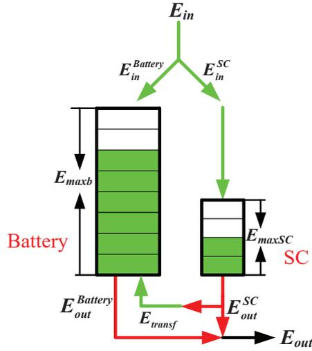
FIGURE 3. Hybrid energy storage unit of EH-based CRSNs nodes
