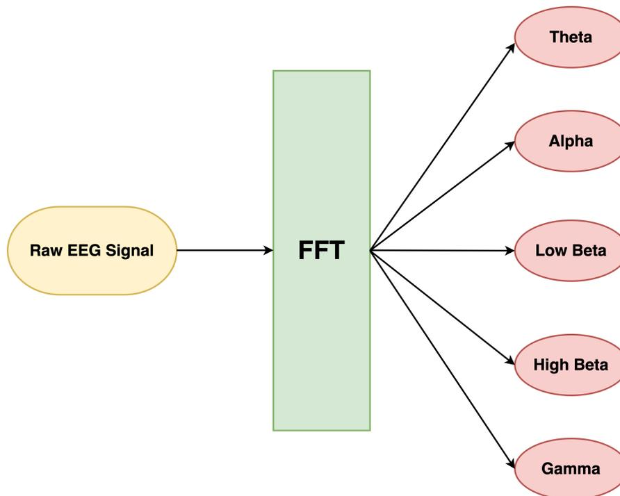
FIGURE 3. FFT feature extraction method.
