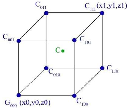
FIGURE 10. Three-dimensional linear interpolation
