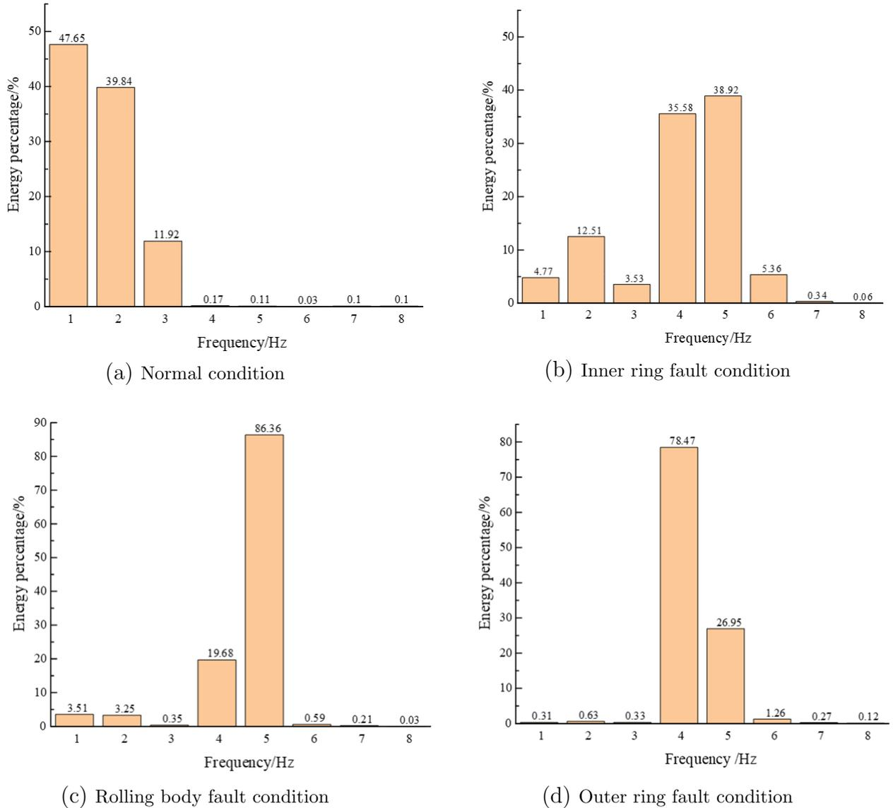
Figure 8. Histogram of the energy share of rolling bearings for different failure states
