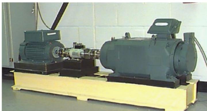
Figure 6. Rolling bearing test bench.
