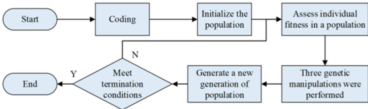
Figure 4. Basic flow of genetic algorithm.
