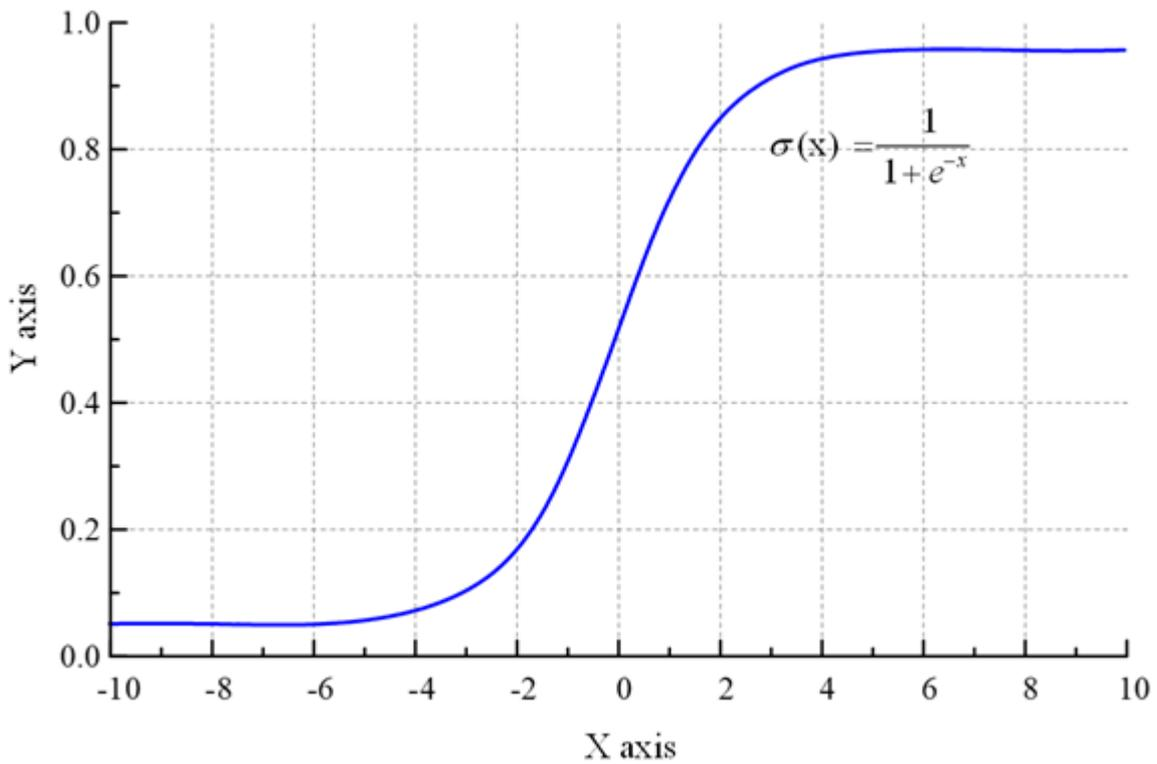
Figure 2. Principle of Sigmoid function.
