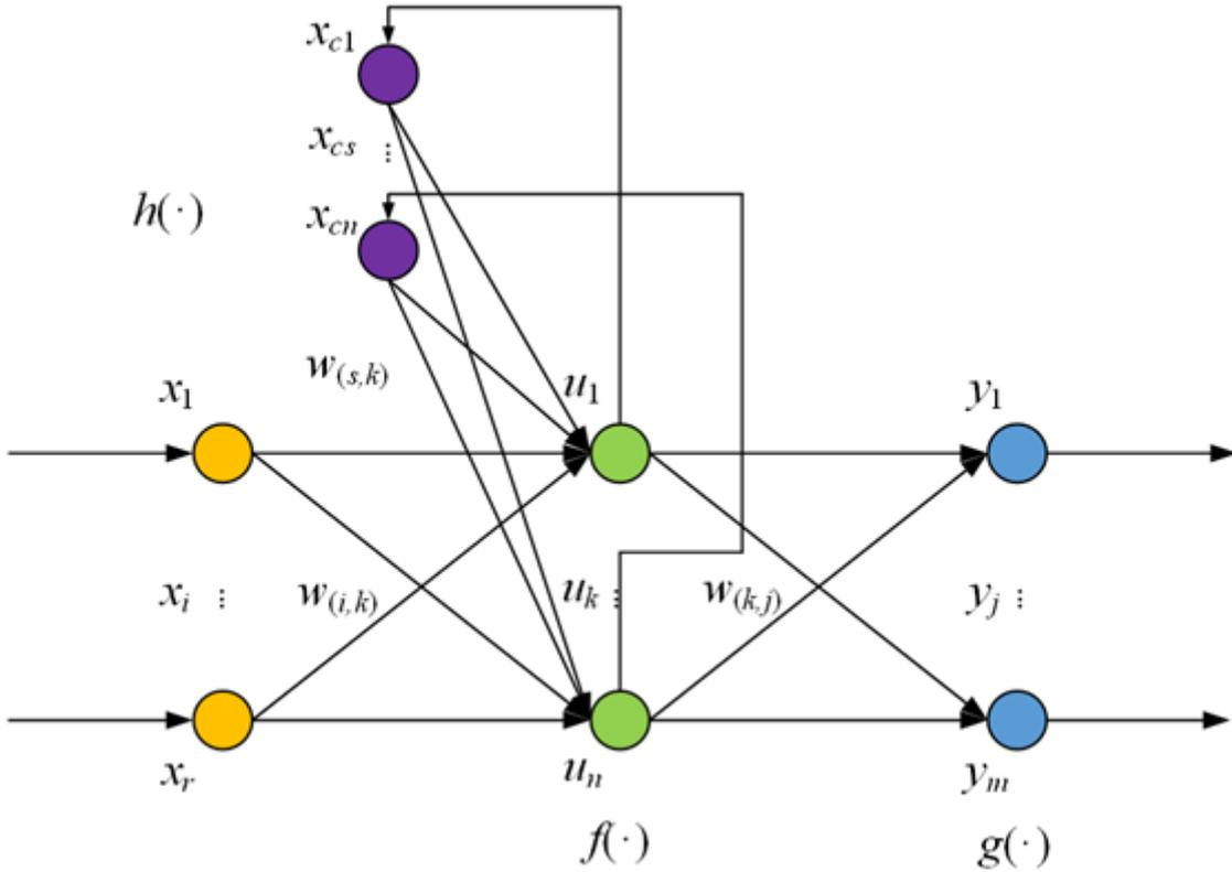
Figure 3. Structure of Elman neural network.
