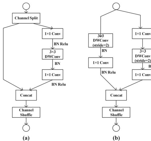
FIGURE 2. ShuffleNetv2 Unit
