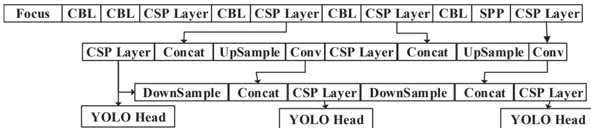
FIGURE 1. The network structures of YOLO v5
