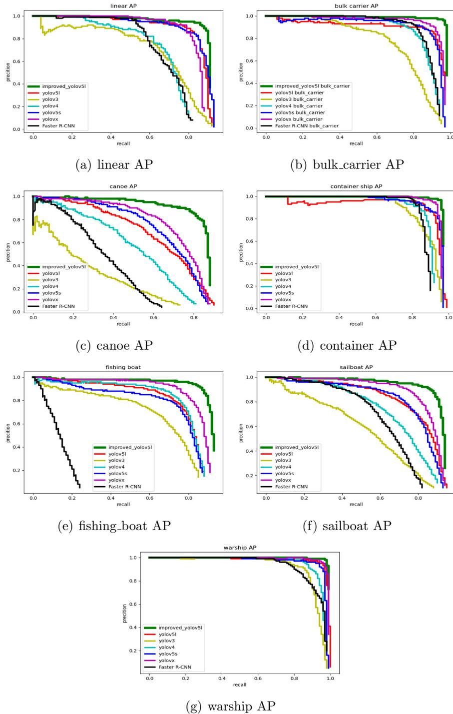
FIGURE 5. Comparison of P-R curves of classical algorithms.
