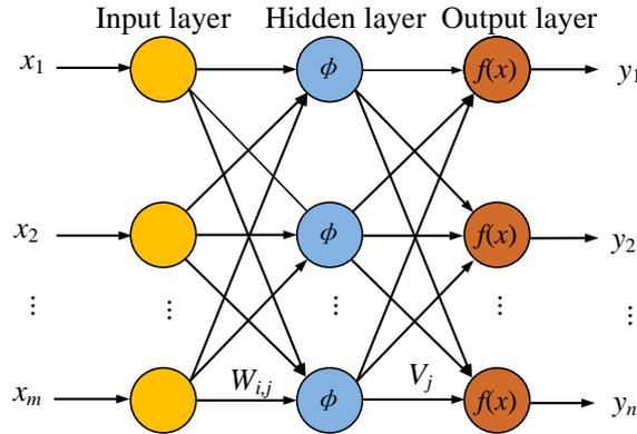
FIGURE 2. Three-layer wavelet neural network
