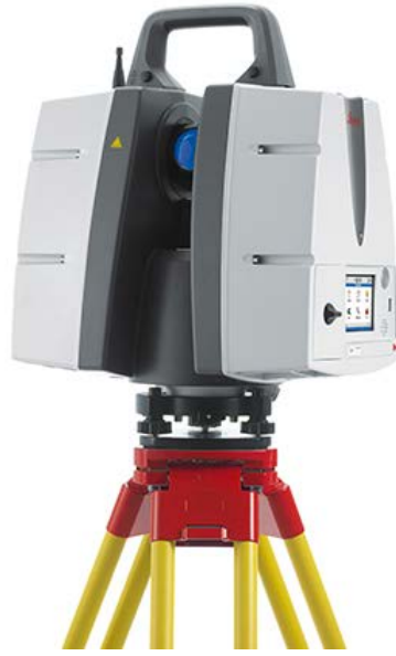
Figure 3. ScanStation P50 remote 3D terrestrial laser scanner
