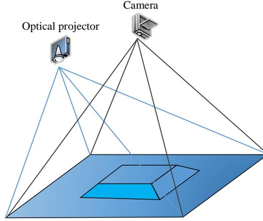
Figure 3. Structured light stereo vision principle
