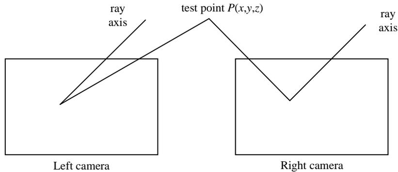
Figure 2. Principle of binocular stereo vision
