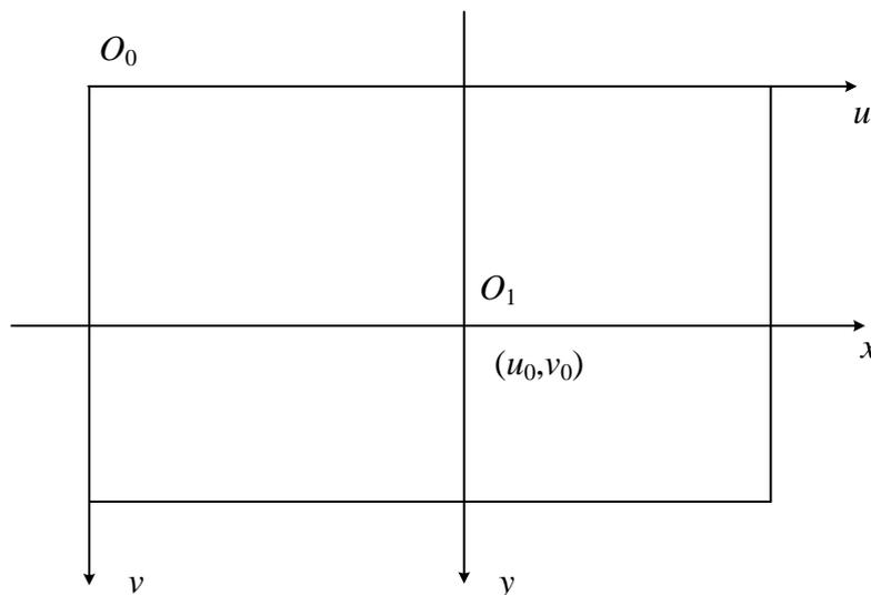
Figure 1. Image coordinate system for camera calibration
