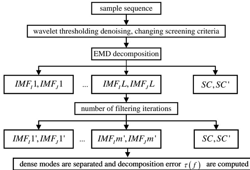
Figure 2. The enhanced process of EMD
