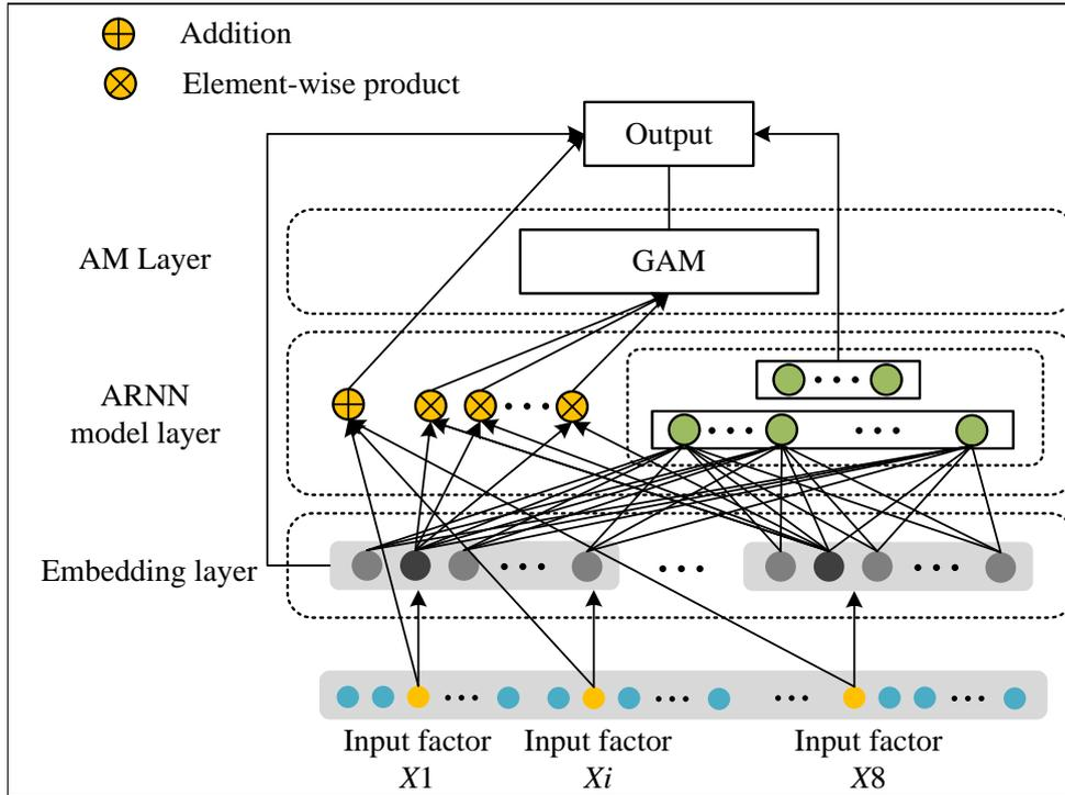
Figure 2. GAM-ARNN based energy efficiency prediction model for assembled concrete buildings
