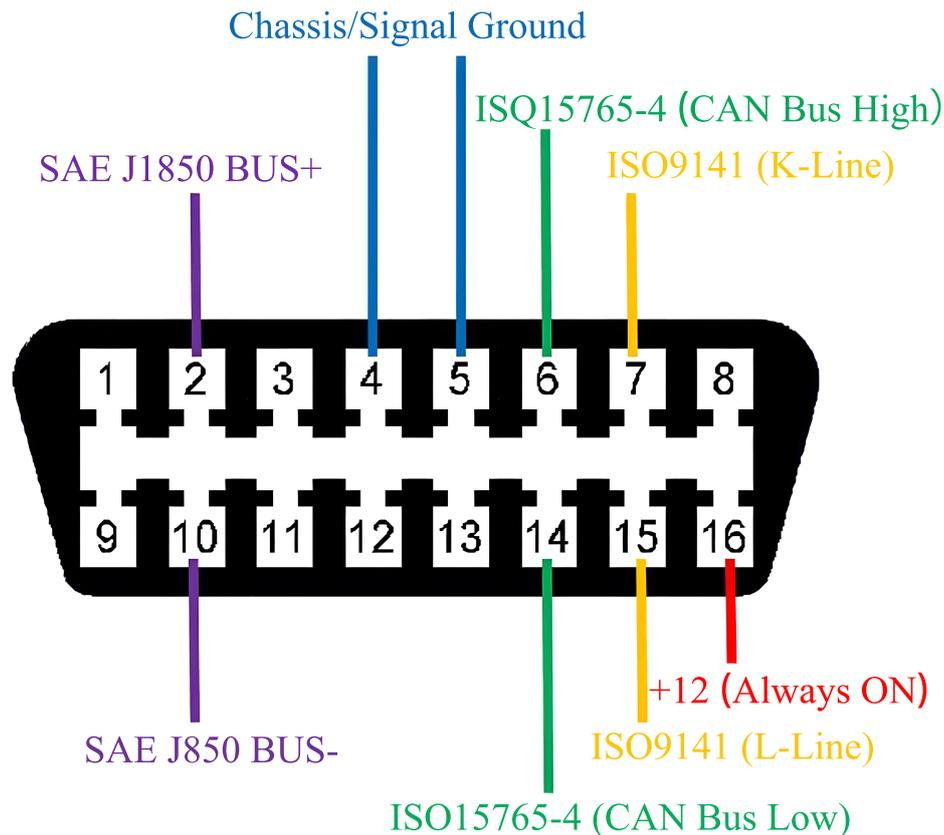
Figure 3. OBD-II Diagnostic Interface Pin Definitions
